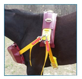
This harness is designed to be placed on a large animal with the intention of providing attachment points for the purposes of maintaining buoyancy. It is not intended, nor strong enough, to perform a vertical lift above the water. The closed cell foam in the saddle of the harness is sufficient to keep the harness from sinking while the chest portion under the neck provides about 32 pounds of buoyancy.
